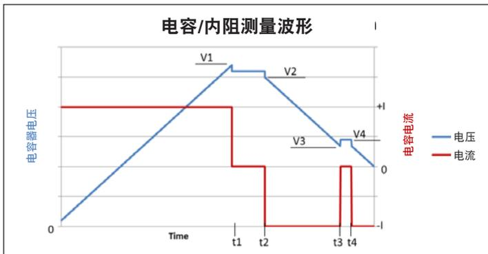
$V1 = V_{rated}$        $t2 - t1 = 15$ 秒      电容 =  $I \times (t3 - t2) / (V2 - V3)$
